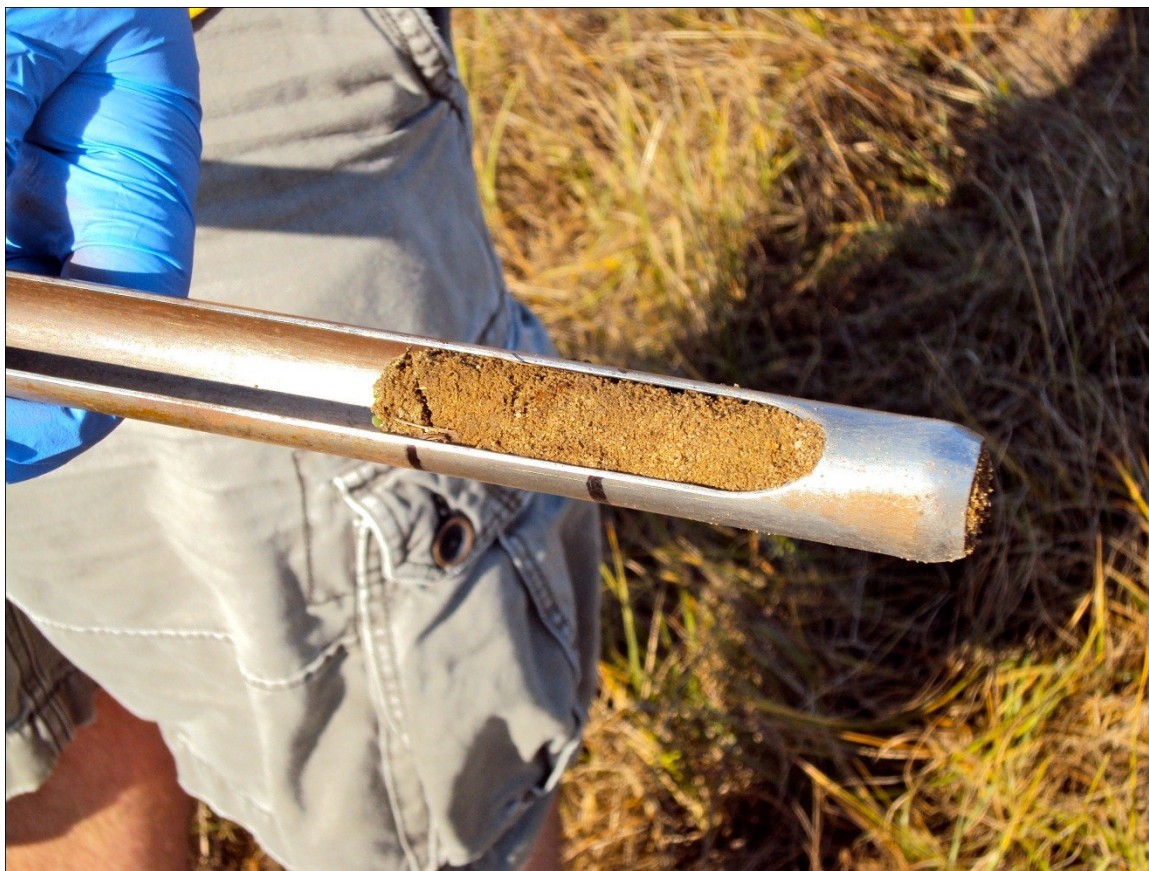
Figure 3-5. Soil corer used to collect Lakeland soil samples at the Range C-62 site on November 13, 2010. Photo taken by Matthew B. Flannigan.
