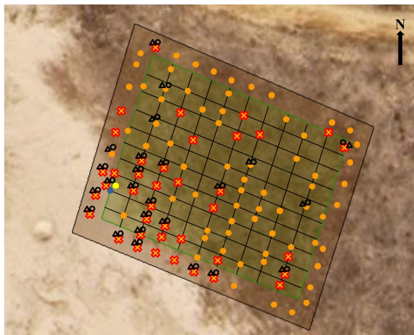
Figure 3-10. Plot #1 detections in soil for the May 24-25, 2010 sampling analyzed with LC/MS. The region shaded is green is the planted portion. The fringe around the edge is unplanted (12 ft wide).
